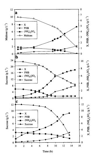
Figure 1: Concentrations of cell dry weight (X), Poly-3-hydroxybutyrate (PHB), growth-limiting substrate ((NH<sub>4</sub>)<sub>2</sub>SO<sub>4</sub>) and carbon sources during discontinuous growth and PHB production experiments with: a: A. latus 1123 on starch hydrolysate (maltose) b: A. latus 1123 on green syrup (sucrose) c: A. latus 1124 on beet molasses (sucrose)
